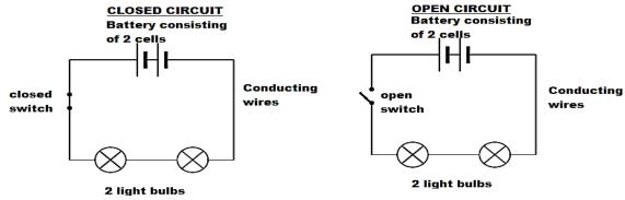
A cell or battery provides the source of chemical potential energy and converts it into kinetic energy caused by the chemical reactions within a cell. An electrical current will flow in a closed system. Electrical charges (electrons) will flow
