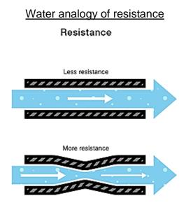
Resistance preventing/ opposing a current through conducting wires.
